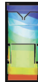
The deformation of the flexure guides is checked with FEM stress simulations
