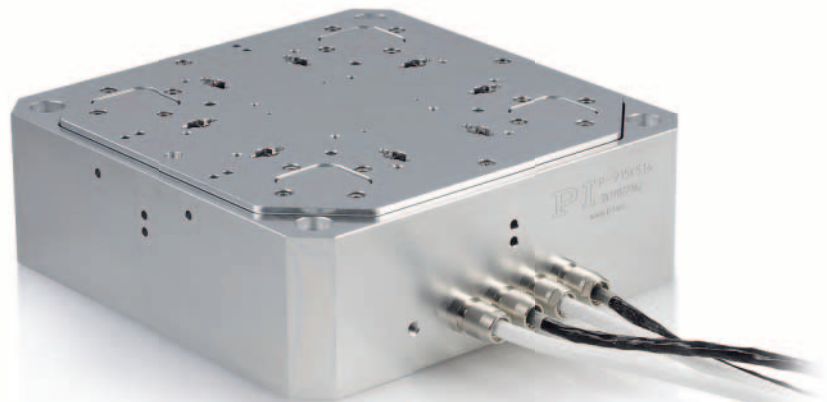
This piezo six-axis stage was developed for Physikalisch-Technische Bundesanstalt (PTB), the German national metrology institute, as object slide in an atomic force microscope (AFM); it is designed for use in UHV. The linear travel ranges are 12 μm × 12 μm × 10 μm; an active correction of the travel accuracy is possible by controlling the tilt axes. With a load of 300 g, it achieves a resonant frequency of over 2 kHz
