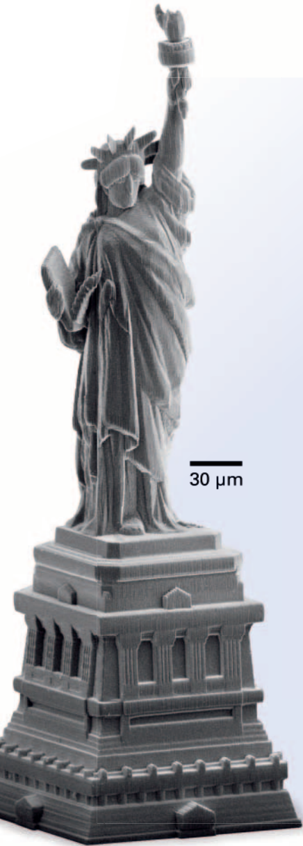
Complex three-dimensional structure: A 300 µm Statue of Liberty was manufactured with 3D laser lithography by Nanoscribe (Photo: Nanoscribe GmbH)
