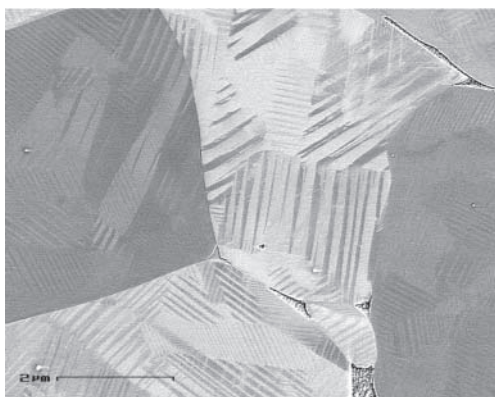
Fig. 2: A cross-sectional view of a ferroelectric ceramic clearly shows the differently polarized domains within the individual crystallites
