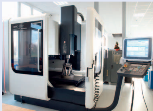
Hexapods in automation. In addition to PLC connection, control over standardized G-Code commands is possible to allow for even higher flexibility
