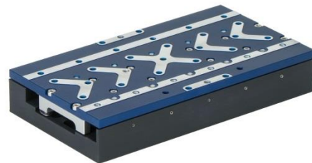
Abb. 8 Driven by PIMag®: Linear stage of the V-508 series based on PI's proprietary linear motor with Halbach array for a particularly flat design with both low weight
