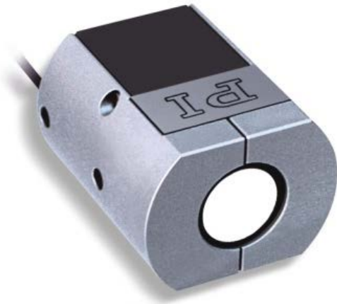
Abb. 5 The piezo-driven tip/tilt platforms are available with tilting angles of up to 3°, which are each offered with position sensors for closed-loop operation or without sensors as fast scanners (Bild: PI)
