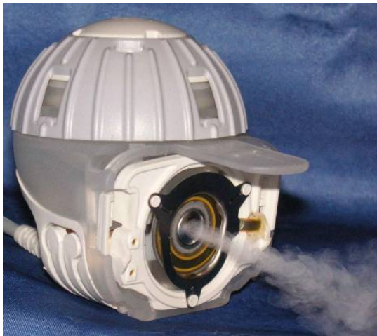
Fig. 8 The aerosol production in the atomizer head of the eFlow® rapid Electronic Nebulizer series uses actuators to generate ultrasonic oscillations (Image: Pari Pharma GmbH)
